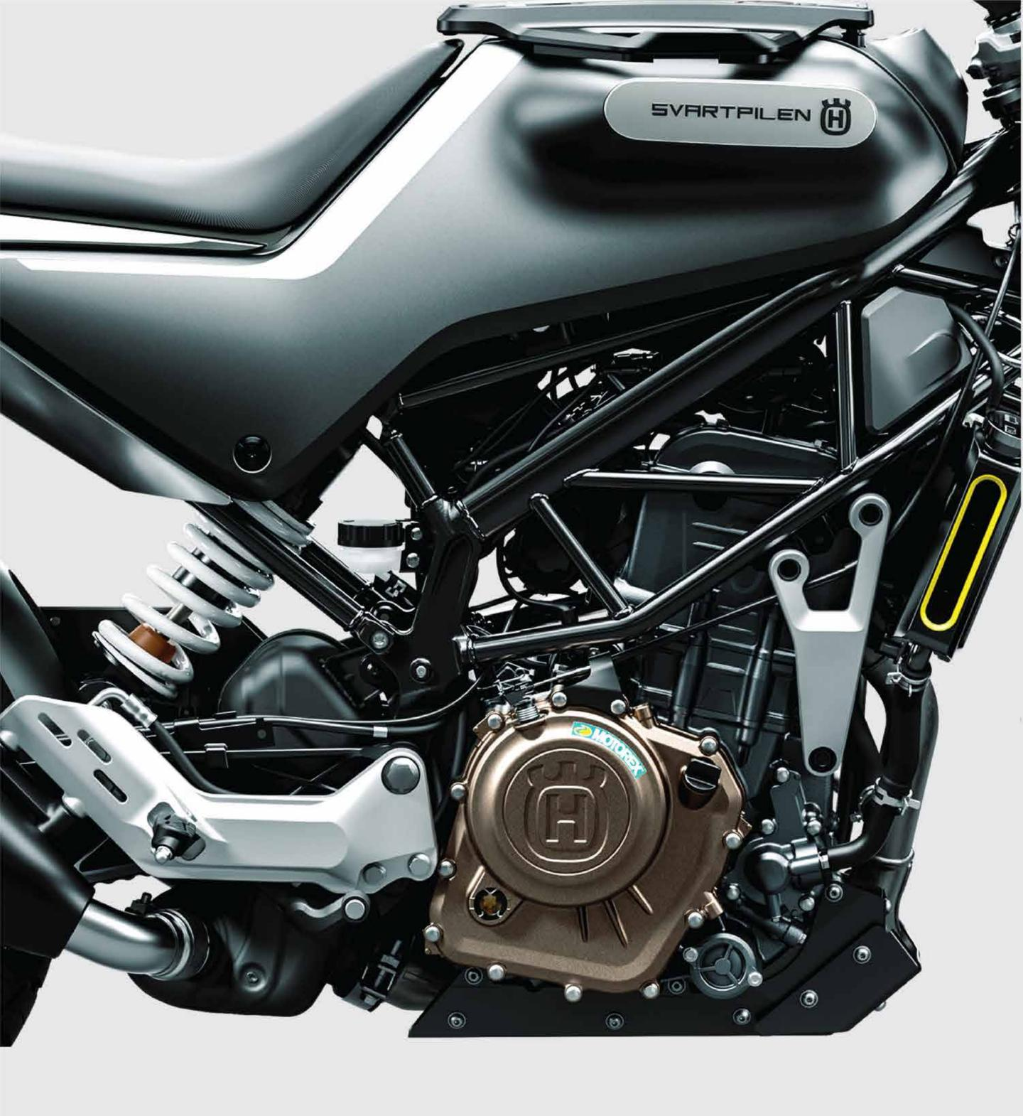
Featuring a sturdy, durable and lightweight steel-trellis frame, upside-down forks, ByBre brakes and a state-of-the-art Bosch ABS system, these machines are designed for a dynamic riding experience every single time you take to the streets. Uninhibited yet always in control
